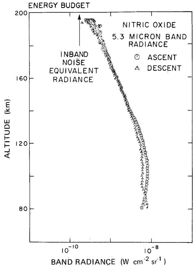
Figure 13-22. Integrated band radiance for the 5.3  $\mu\text{m}$  NO signal observed in the Energy Budget campaign during ascent and descent as a function of tangent height.
