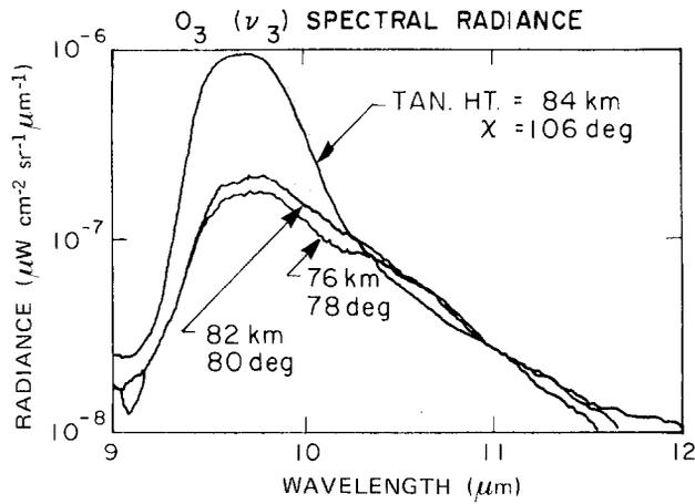
Figure 13-11. 9.6  $\mu\text{m}$  ( $\nu_3$ ) ozone spectrum at 80 km tangent height for different solar elevation angles. The signal for wavelengths longer than 10.2  $\mu\text{m}$  shows no diurnal variation..
