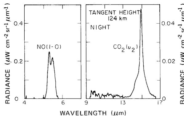
Figure 13-7. Nighttime radiance seen by the long wavelength SPIRE spectrometer as function of wavelength at 124 km tangent height. NO ( $1 \rightarrow 0$ ) band at 5.3  $\mu\text{m}$  and  $\text{CO}_2$  ( $01101 \rightarrow 00001$ ) band at 15  $\mu\text{m}$  are the only reproducible spectra seen. Scale for the NO band is 10 times larger than that for  $\text{CO}_2$  band. (Daytime results were essentially the same.)
