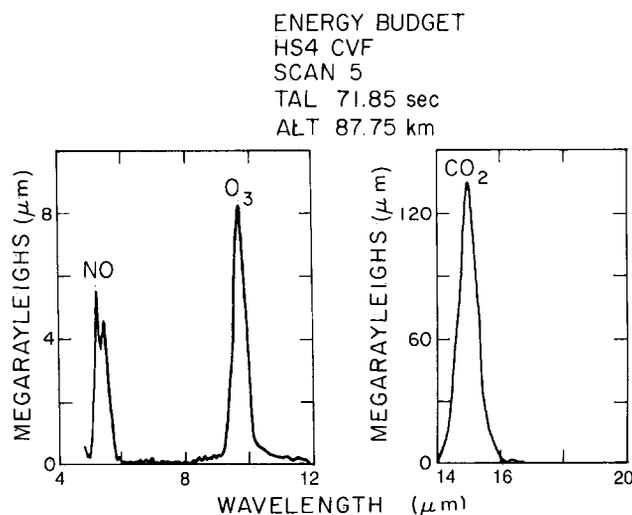
Figure 13-2. Plot of radiance vs wavelength from the zenith looking CVF "Energy Budget" rocket at 87.75 km altitude. The signal from  $\text{CO}_2$  at 15  $\mu\text{m}$  is at least an order of magnitude larger than that from NO at 5.3  $\mu\text{m}$  or ozone at 9.6  $\mu\text{m}$ .
