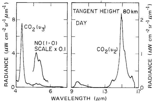
Figure 13-8. Daytime signal from the long wavelength SPIRE spectrometer as function of wavelength at tangent height of 80 km. The 15  $\mu\text{m}$  CO<sub>2</sub> and 5.3  $\mu\text{m}$  NO signals are about the same as in Figure 13-9 (nighttime). The 4.3  $\mu\text{m}$  CO<sub>2</sub> signal is enhanced and 9.6  $\mu\text{m}$  O<sub>3</sub> signal is reduced over nighttime values (Figure 13-9).
