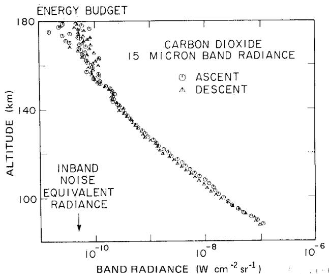
Figure 13-6. Integrated band radiance around 15  $\mu\text{m}$  observed by zenith-looking Energy Budget rocket during ascent and descent as function of altitude.
