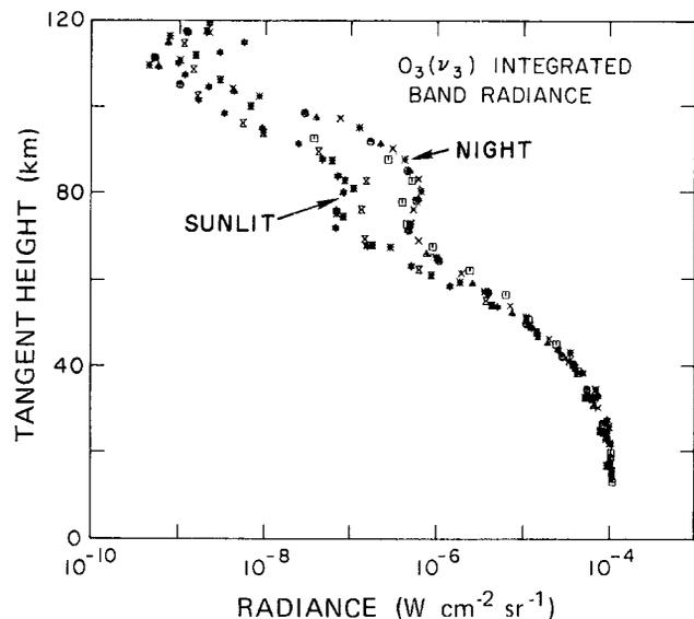
Figure 13-10. 9.6  $\mu\text{m}$  ( $\nu_3$ ) ozone (19.20–10.50  $\mu\text{m}$ ) band radiance as function of tangent height. Note stronger nighttime radiance and peak around 80 km. A terminator crossing is evident in scan 1 ( $\square$ ) where the radiation decreases by an order of magnitude from 85 to 90 km.
