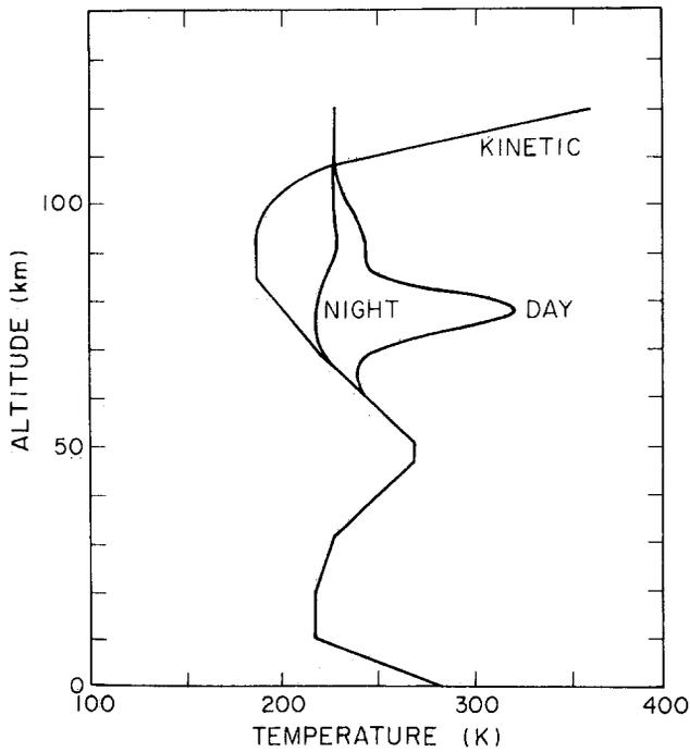
Figure 13-23. Daytime and nighttime vibrational temperatures of  $\nu_3$  mode of ozone as function of altitude [Degges and Smith, 1977].
