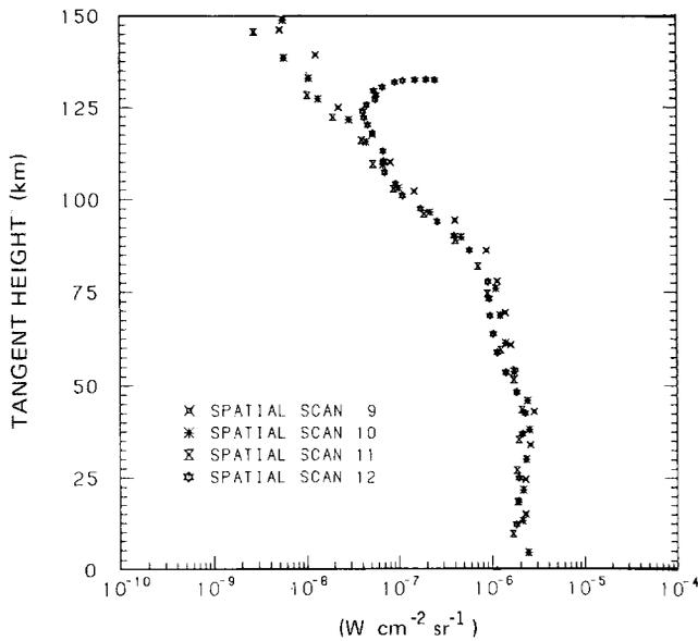
Figure 13-12. Daytime integrated 4.3  $\mu\text{m}$  band radiance observed by short wavelength SPIRE spectrometer as function of tangent height. Larger signal in scan 12 is due to the fact that a deliberate effort was made in this last scan to test the telescope.
