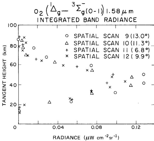
Figure 13-16. Integrated (1.51–1.65  $\mu\text{m}$ )  $\text{O}_2$  ( $1^1\Delta_g$ ) radiance at 1.58  $\mu\text{m}$  as function of solar elevation angle. Peak signal around 40 km shows inverse correlation with solar elevation ( $\chi$ ) angle.
