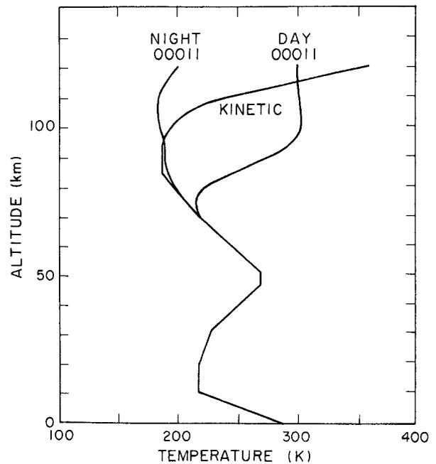
Figure 13-18. Daytime and nighttime vibrational temperatures of asymmetric stretch of  $\text{CO}_2$  as function of altitude. Kinetic temperature is also plotted for comparison [Degges and Smith, 1977].
