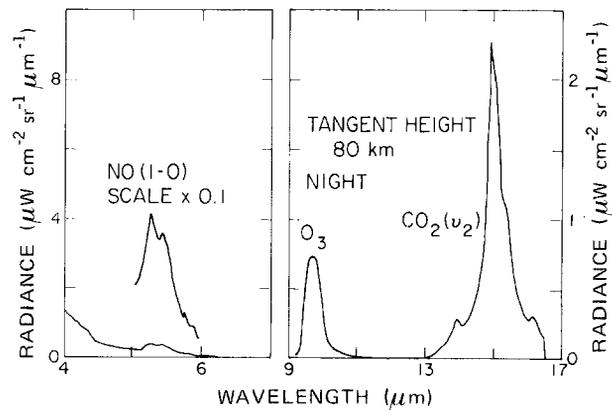
Figure 13-9. Nighttime signal for long wavelength SPIRE spectrometer as function of wavelength at tangent height of 80 km. Notice appearance of O<sub>3</sub> ( $\nu_3$ ) signal. The apparent signal in the 4–6  $\mu\text{m}$  region is due to dielectric relaxation response of the detector to the 15  $\mu\text{m}$  radiation. The 5–6  $\mu\text{m}$  region has been magnified 10-fold to highlight the NO spectral features.
