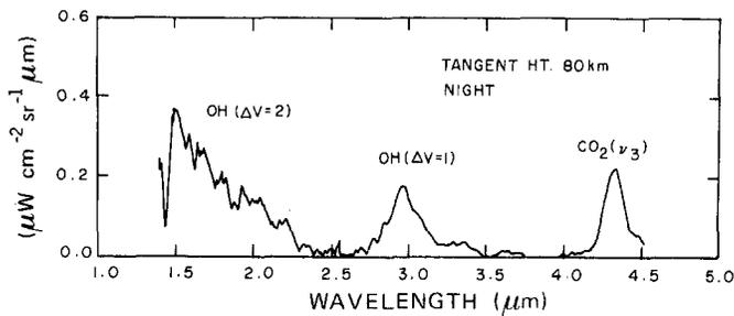
Figure 13-15. The nighttime signal from near infrared spectrometer as function of wavelength. Notice the progression of OH overtone bands ( $\Delta v = 2$ ) between 1.5–2.4  $\mu\text{m}$  and the OH fundamental bands ( $\Delta v = 1$ ) peaked at about 3  $\mu\text{m}$ . The fluorescent emission at 4.3  $\mu\text{m}$  is shown here without the effects of the dielectric relaxation problem encountered in the long wavelength spectrometer.
