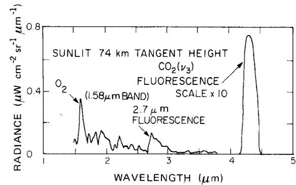
Figure 13-14. The daytime signal from near infrared spectrometer at 74 km tangent height. The nighttime  $\text{OH}$  radiation is reduced.  $\text{O}_2(a\Delta_g, v=0) \rightarrow {}^3\Sigma_g^-(v=1)$  radiation appears at 1.58  $\mu\text{m}$ . The 2.7  $\mu\text{m}$  radiation is fluorescence signal from  $\text{CO}_2(\nu_1 + \nu_3$  combination bands) and  $\text{H}_2\text{O}(\nu_1$  and  $\nu_3$  bands).
