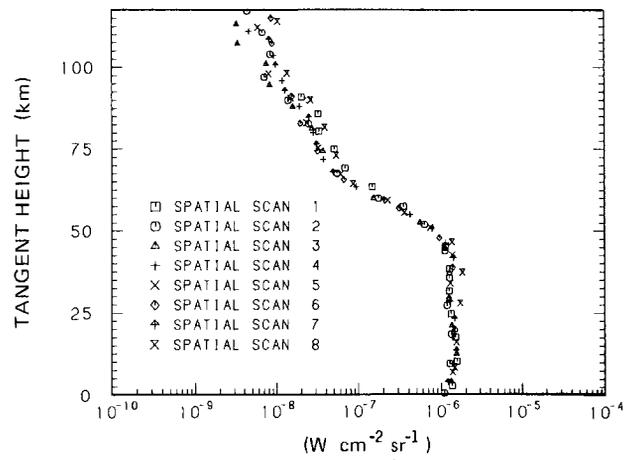
Figure 13-13. Nighttime integrated 4.3  $\mu\text{m}$  band radiance observed by short wavelength SPIRE spectrometer. Notice much faster decrease of the signal above 70 km tangent height than for the daytime case.
