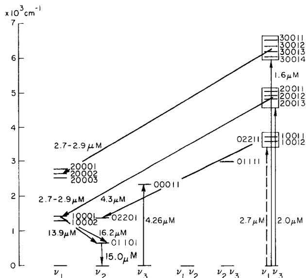
Figure 13-1. The energy levels of carbon dioxide. The lowest levels of bending mode and asymmetric stretch, which lead to transitions at  $15.0$  and  $4.26 \mu\text{m}$ , are shown. Also shown are the upper and lower levels for some of the important transitions observed in the infrared airglow of the earth's atmosphere. The notation in the figure is the same as in AFGL line tape [Rothman and Young, 1981]. (Reprinted with permission from Pergamon Press Ltd. © 1981.)
