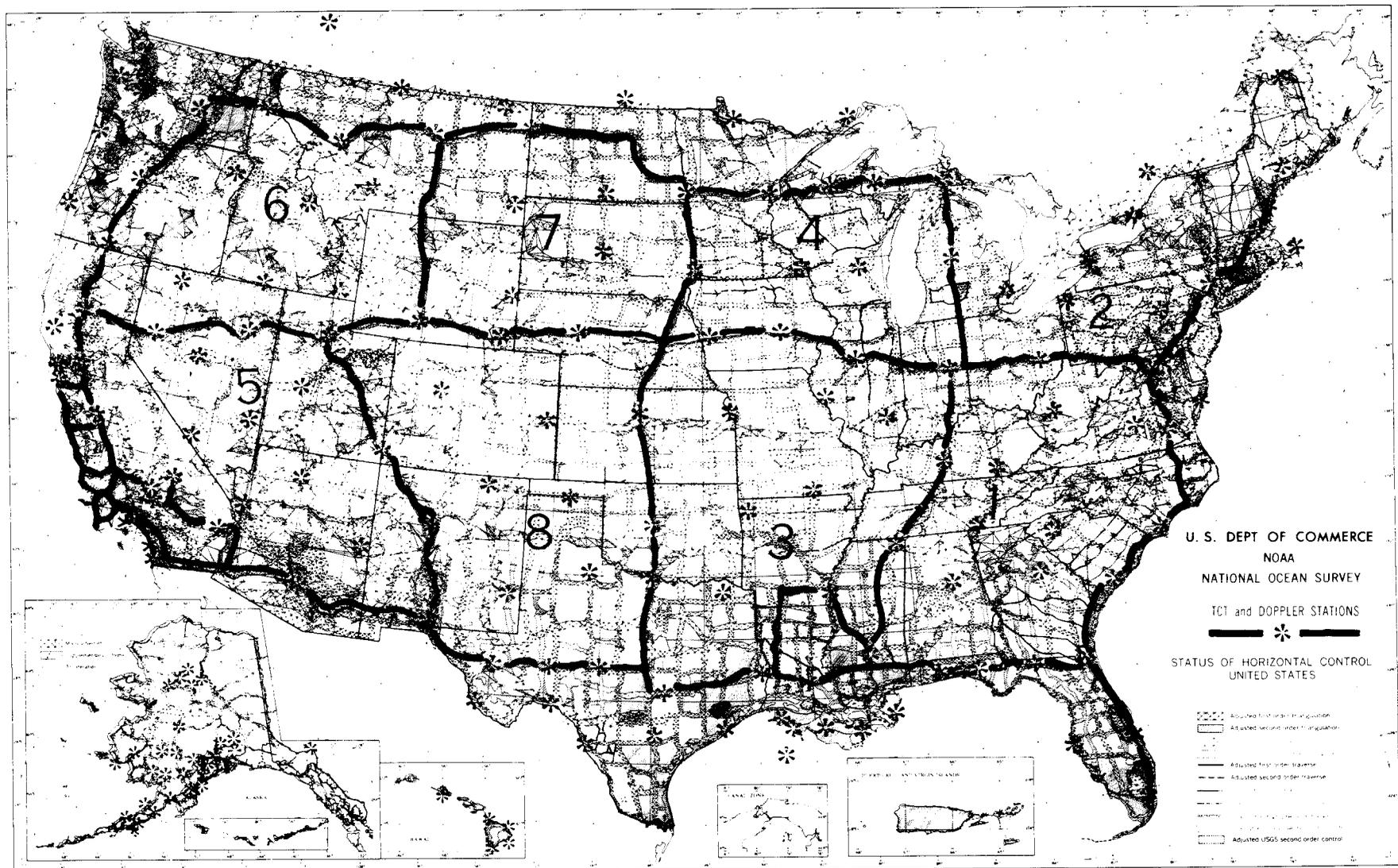
Figure 24-2. Status of horizontal control in the United States [NRC, 1978].
