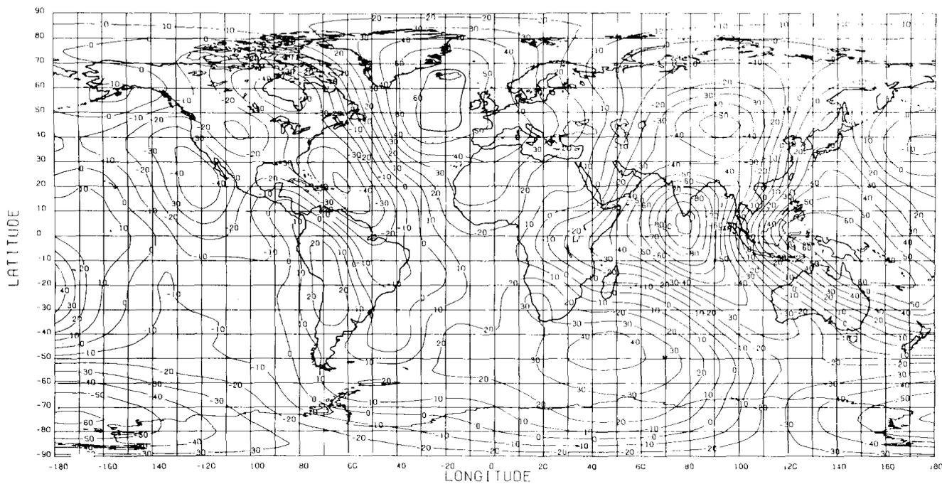
Figure 24-5. Long-wavelength geoid undulation contours (contour interval = 10 m) from (14.14) solution using weighted GEM 10 coefficients and altimetric data; reference flattening =  $1/298.25$  [Hadjiageorge, 1981].
