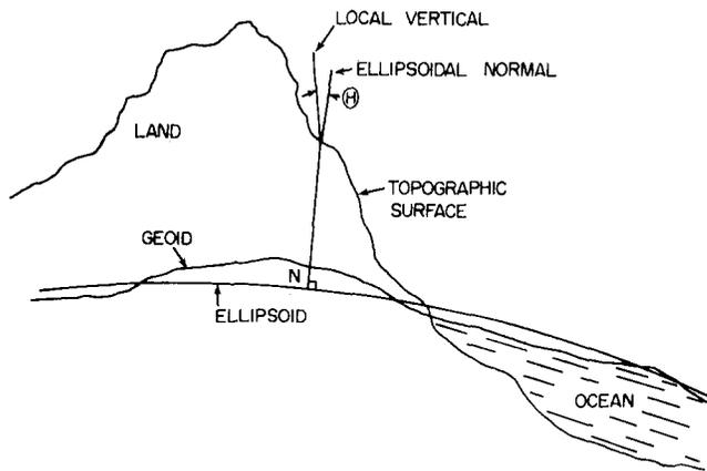
Figure 24-1. The relationship between the geoid and the ellipsoid.
